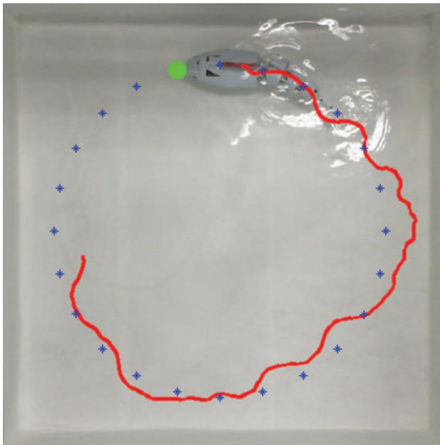
**Figure 9.** The robotic fish swimming in a circular path utilizing a PID controller algorithm. The waypoints are indicated by the blue diamond markers. The next waypoint in the snapshot for the robotic fish is indicated by the green circle marker. The path taken by the robotic fish in 30 s is indicated by the red line.
