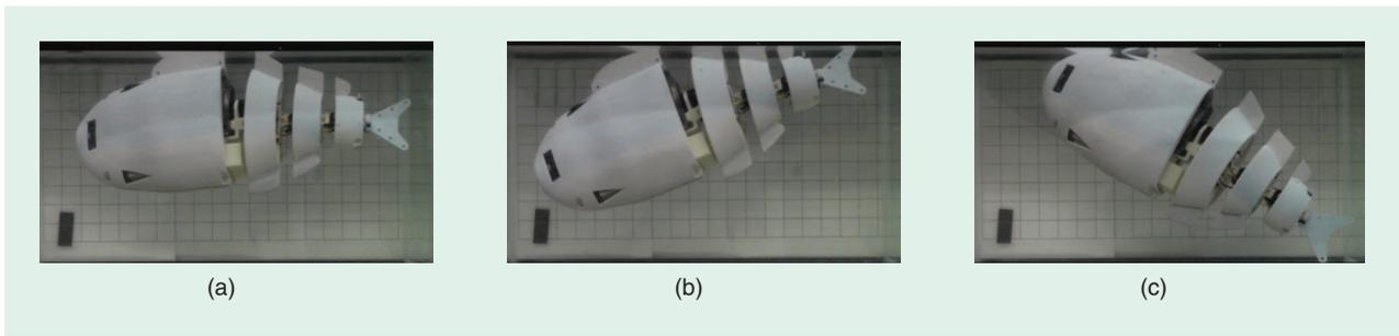
**Figure 7.** The pitch performance for the robotic fish. The robotic fish can be set to (a) neutral pitch, (b) maximum downward pitch, or (c) maximum upward pitch.
