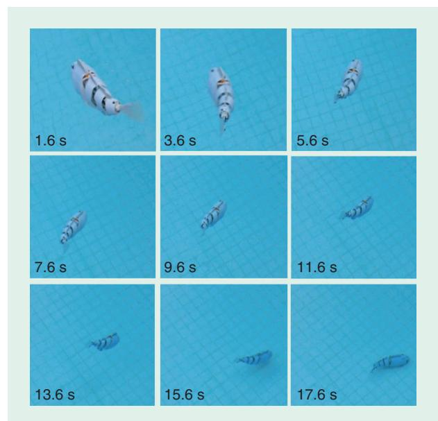
**Figure 8.** A sequence of snapshots of the robotic fish during the diving test.
