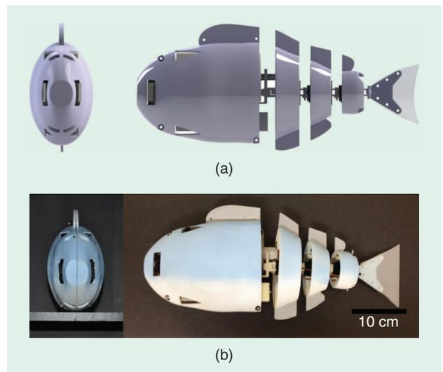
**Figure 1.** The front and side views of the (a) computer-aided design (CAD) and (b) physical prototype of the robotic fish.
