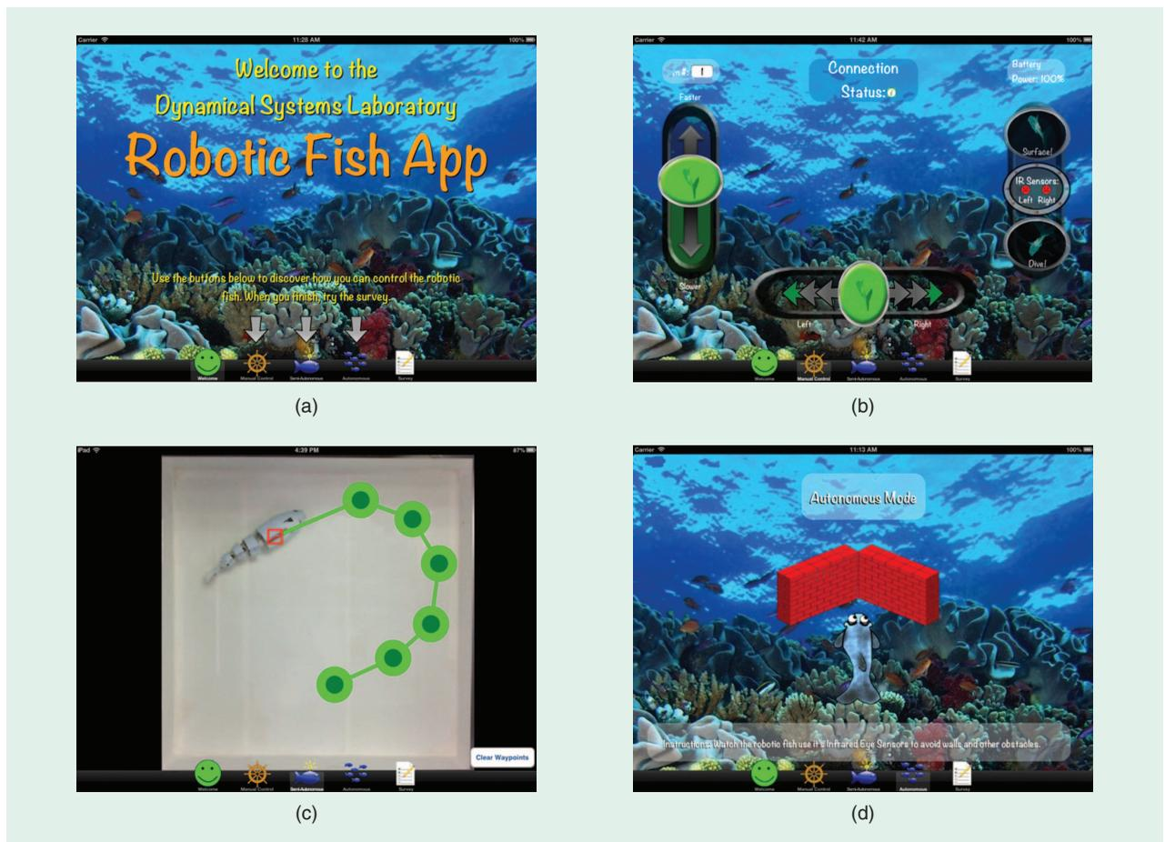
Figure 5. Screenshots of the iDevice app showing the (a) welcome screen, (b) manual mode, and (c) and (d) autonomous mode.
