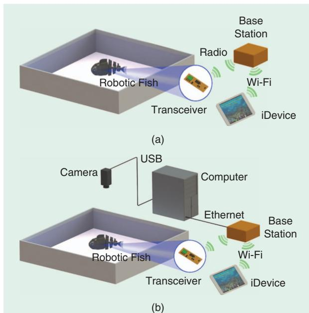
**Figure 4.** A schematic representation of (a) the communication protocol between the robotic fish and the iDevice for the manual and autonomous modes and (b) the additional components required for the experimental setup in the semiautonomous mode.
