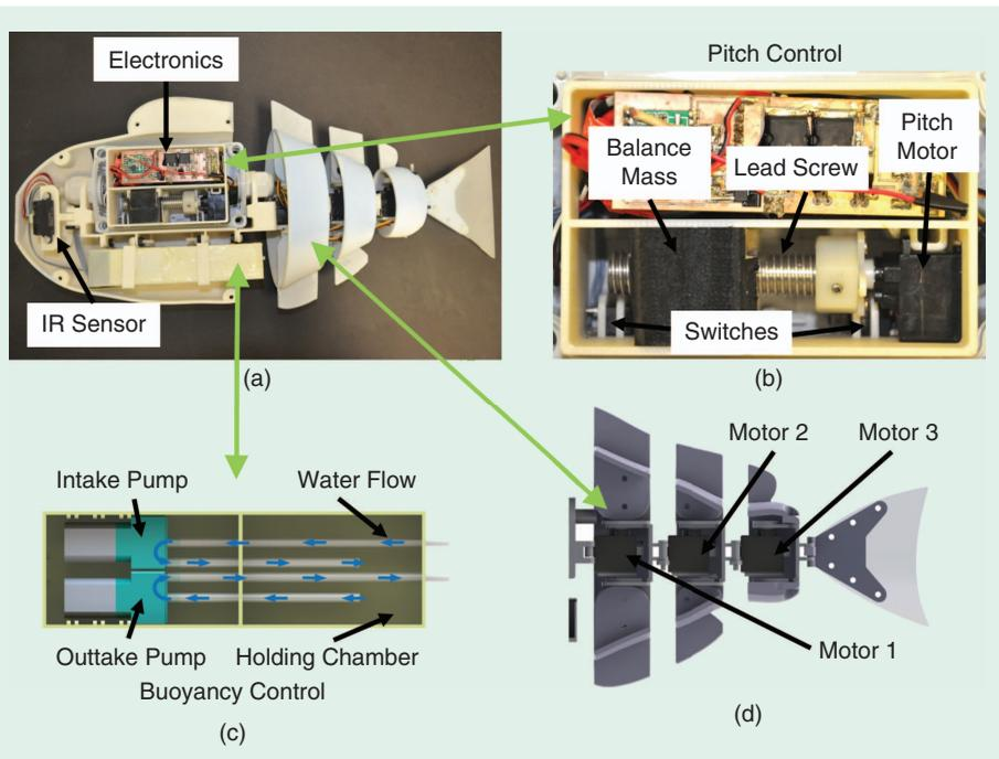
**Figure 2.** (a) The waterproof housing displaying the exposed electronics, sensors, and pitch control system. (b) The pitch control motor, lead screw, balance mass, and limit switches. (c) A CAD illustration of a cutaway top view of the buoyancy control tank, water pumps, and holding chamber. (d) A CAD illustration of a cutaway view of the robotic fish tail including the servomotors, links, and caudal fin.
